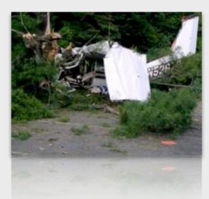
Federal safety officials made their final determination on what may have been the contributing factors of the crash. Officials concluded the plane lost power because of the lack of oil from a leak. In addition the mechanic's sign-off and release of the airplane without performing the required engine run-up following an annual inspection.
